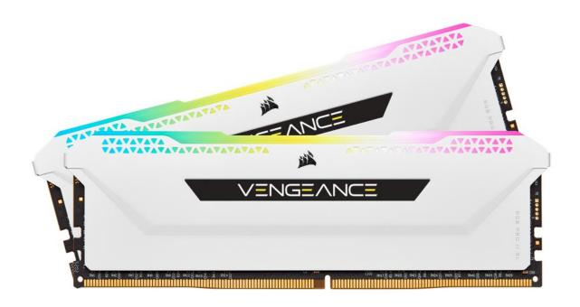
At 44mm tall, VENGEANCE RGB PRO SL's compact form-factor enables compatibility with a multitude of CPU cooler options, including dual-fan AIO liquid CPU coolers and many air coolers such as the CORSAIR A500. Ten individually addressable RGB LEDs per module are
