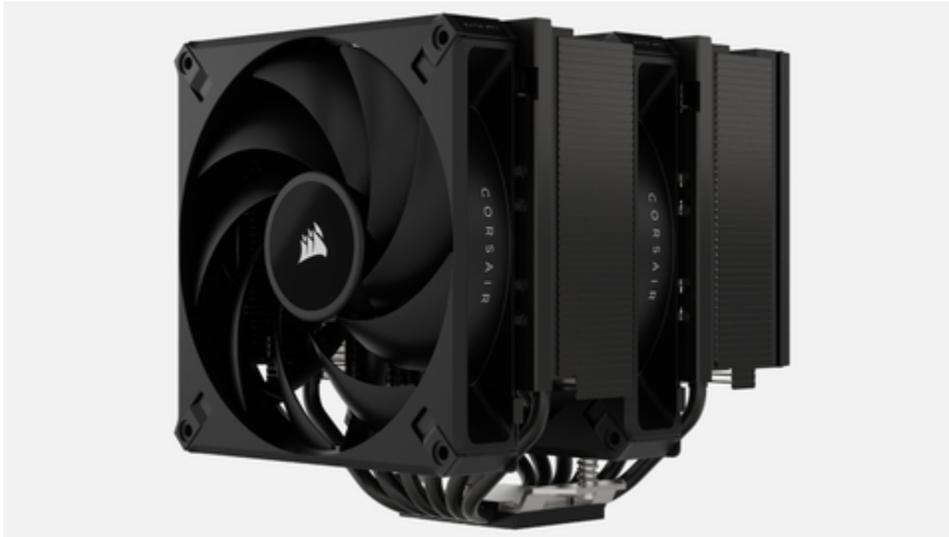
At the heart of the A115 are six 6mm heat pipes and a high-efficiency copper cold plate, capable of handling CPUs with up to 270W TDP. The slightly convex shape of the cold plate optimizes contact with the CPU, ensuring maximum thermal transfer and stability. After absorbing heat, 90 nickel-plated cooling fins provide a substantial 1.69m<sup>2</sup> surface area for rapid heat dissipation.
