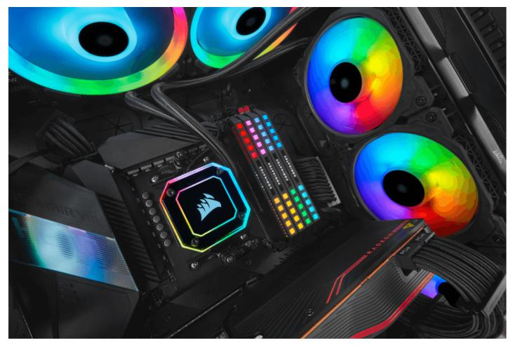
The excellent cooling provided by iCUE ELITE CAPELLIX coolers starts with a high-performance centrifugal pump, delivering a flow rate of up to 0.82L/min while generating less than 20 dBA, for extreme cooling with low noise. A split-flow copper cold plate rapidly absorbs heat from your CPU, while powerful ML RGB Series fans dispel that heat after it is carried to the radiator, utilizing magnetic levitation bearings to spin at up to 2,400 RPM with precise PWM control.
